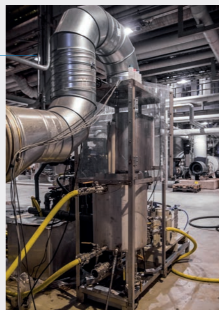
Figure 2. ANDRITZ began pilot plant testing of Lignin Recovery alternative concepts in 2010. Shown here is the portable pilot plant that can be easily transported to mills.
