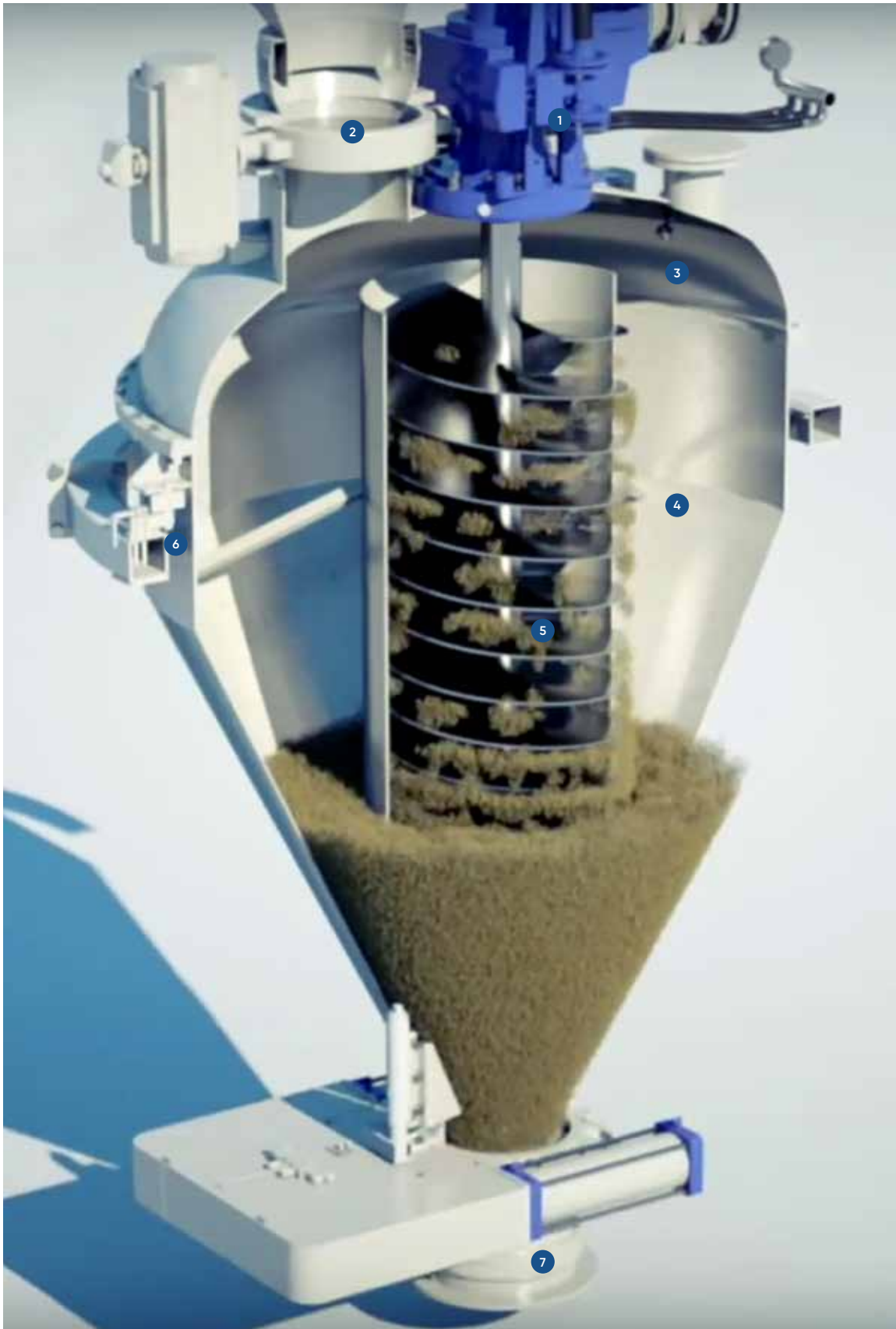
1 Gear motor 2 Inlet valve 3 Spray nozzles 4 Barrel 5 Screw 6 Load cells 7 Discharge valve
